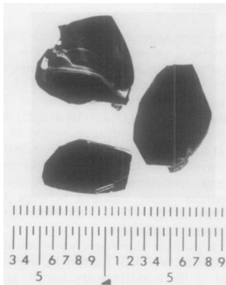
FIG. 1. Photographs of Nb-doped iron oxide single crystal platelets 6 \times 5 \times 1 mm.
